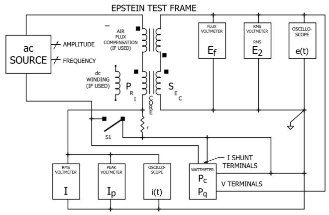
NOTE 1—The ac source terminals must "float" to prevent ground loop currents. If the wattmeter has a common connection between its V and I terminals, the rest of the circuit must be connected so as to prevent shorting.
